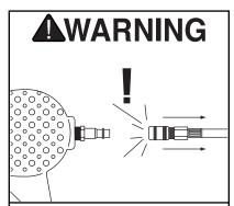
Always disconnect air from the nailer whenever servicing! During maintenance, a nailer connected to air may fire accidentally, causing serious personal injury!
